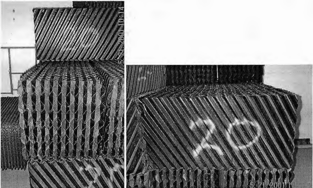
Figure A2. TFs 60° crossflow media with a specific surface area of 30 \text{ ft}^2/\text{ft}^3 .
